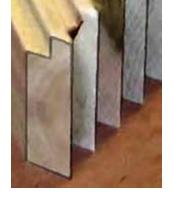
An inside edge lip is needed on all sides and ends so the table top can be dropped into place and glued. Cut this before you assemble the box. Also consider using a small roundover bit on the outside edge for splinter control and to reduce elbow, chin, and head dents later...
